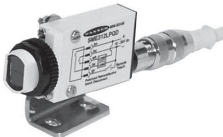
The HQC-100-PCT-LR is a compact, long range retro-reflective Photocell which is used for non-contact triggering of the HQC marking cycle. This unit has an effective range up to 10 feet and is rated for harsh environments and suitable for installation in wet areas. Body Dimensions: 2.6” x 1.21” x 0.48”.
