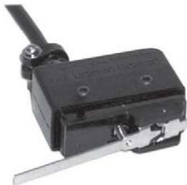
The HQC-100-MST Micro-Switch is a contact trigger used to initiate the print cycle of the HQC. This unit is permanently mounted to the production line and has a 2.5” long trip lever with a low (2.5 Oz.) operating force. Body Dimensions: 2.1” x 1.55” x 0.84”.
