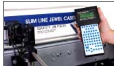
each module together which allows the hand held controller to network all of the print heads. A longer cable is used to connect the modules to the printers on the next production line in the manufacturing area.
