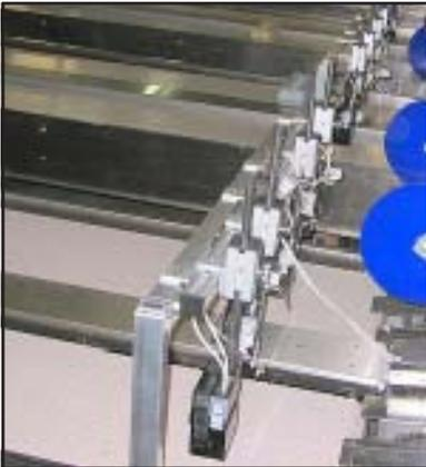
**The Mounting Bracket** will hold up to 4 separate print head modules at once. A small RS 485 data cable is used to connect each module together allowing the hand held controller to network all of the print heads. When using multiple print heads, each print head module has a discreet address so you can identify them for message entry. The hand
