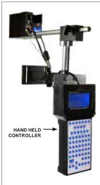
*This system comes equipped* with a hand held controller with tactile keypad for message entry, and a LCD graphics display, printhead module, breakaway mounting bracketry and four character heights in the Arial style font, 1/2", 7/32", 1/8" and 3/32". The controller is also capable of controlling up to 32 individual printhead modules.
