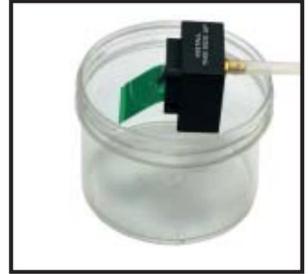
7 - Press the PUMP START button and the pump will begin to run. You may need to lift the ink reservoir above the height of the pump module until the ink begins filling the ink tubes on the Coder output side of the pump.
