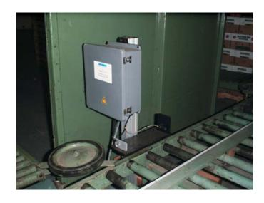
Both the marking and the scanning system require 115 VAC, 60 Hz power and an electrical interface with the parent equipment for operation. The marking system requires 80 psi clean, dry, compressed air. A single 64 oz. gravity feed ink reservoir and an air distribution manifold can be used to supply up to 4 markers.
