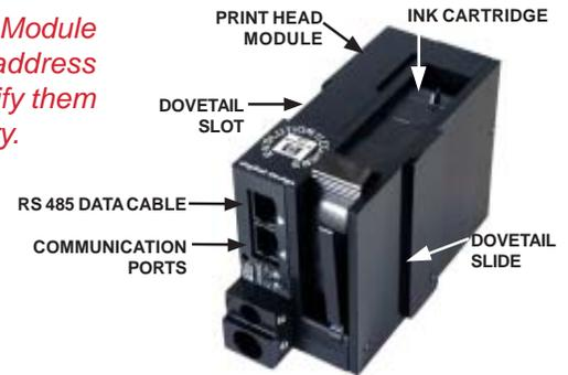
**The Mounting Bracket** will hold up to 4 separate print head modules at once; a small RS 485 data cable is used to connect each module together which allows the hand held controller to network all of the print heads. The controller has the capability of controlling up to 32 individual print head modules. A longer cable is used to connect the modules to the printers on the next production line in the manufacturing area.
