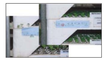
As the trays arrive at the end of the conveyor, the operator simply has to place all the trays with the same symbol on the same pallet for shipment to the customer.
