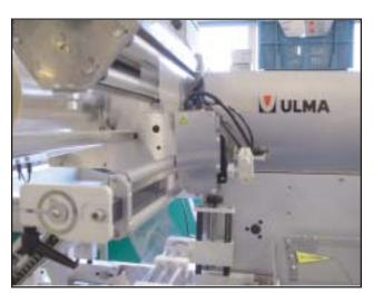
A very large vegetable packing company uses 25 Hot Quick Coders on their ULMA horizontal flow wrappers to mark packing date codes on unimprinted plastic bags of fresh cut vegetables. These code dates are for internal use for tracking inventory freshness. The company packs 280 different products at a rate of 3 million bags per week.
