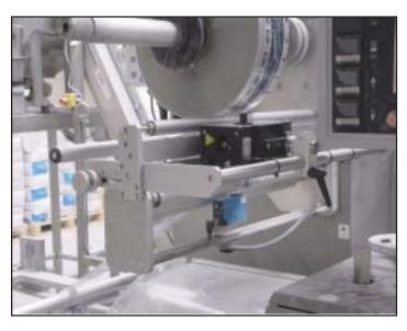
A candy manufacturer uses a Klockner-Hansel horizontal flow wrapper to individually pack large gum balls in a colored plastic film. The Kortho Hot Quick Coder is used to apply 3 lines of 2.5mm code to the film including product code, manufacturing date and expiration date.
