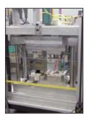
Electronic assemblies are manually placed in a fixture by the inspection system operators. Assemblies which pass all inspection criteria are automatically marked with a 6mm diameter round spot mark. The yellow hot ink rolls provide a high contrast mark on the black plastic components. The instant drying marks enable immediate handling by the system operators.
