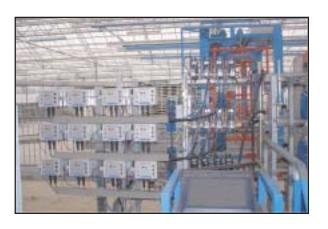
A producer of seedlings uses an automated processing system to pick and sort inventory for customers orders. When the various trays of seedlings are picked from the greenhouses, a bar code containing customer order information is applied to each tray. All of the trays are automatically routed to one of three conveyors for transport to area where the trays are palletized for shipment.
