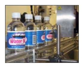
The date codes in this application are applied horizontally on the top edge of the labels on some of the production and directly on the crown of the bottles during production of unlabeled products. The codes applied by the Kortho Hot Quick Coder dry instantly even when the surface of the bottle is slightly wet.
